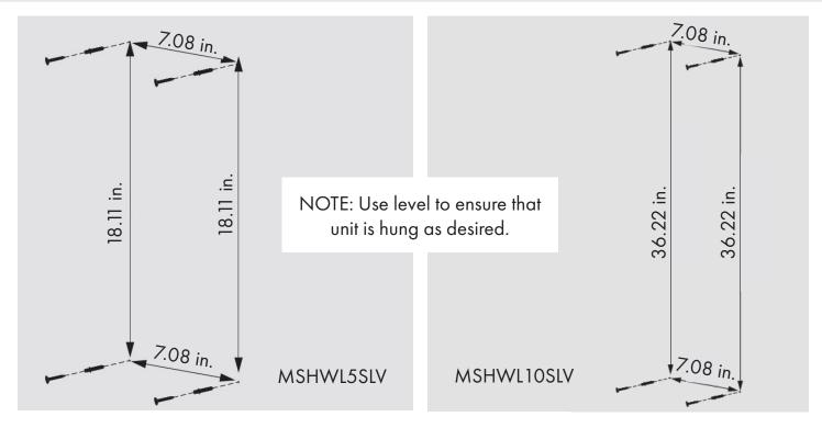
1a. Measure and mark wall at desired location by using the illustration above or by holding unit against the wall at desired height and marking wall through the screw holes.
